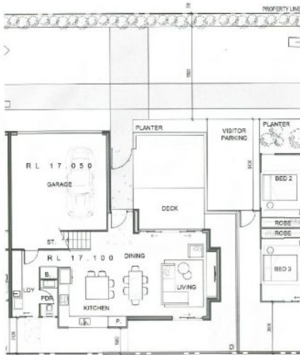
ground floor plan | area 69m 2 ground floor garage | area 36m 2 floor plan - unit 2 1:100
